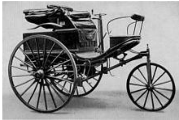
1885 - Benz Patent Motorwagen First production internal combustion engine (ICE) car
